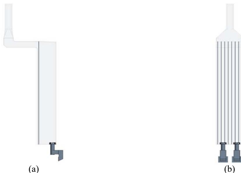
Figure 7: CFD model of 2 burners in a cracking furnace simulator: (a) side view, (b) front view.
